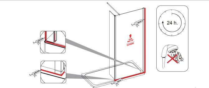
Before sealing make sure all surfaces are clean, dry and free from any residue such as grout. Use quality silicone sealant and applicator gun to fnish the wetroom panels.
