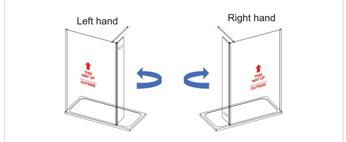
Step 1 – Remove swivel panel from packaging. Install the swivel panel in required orientation. Product is reversible and no brackets need to be removed to change handing.
